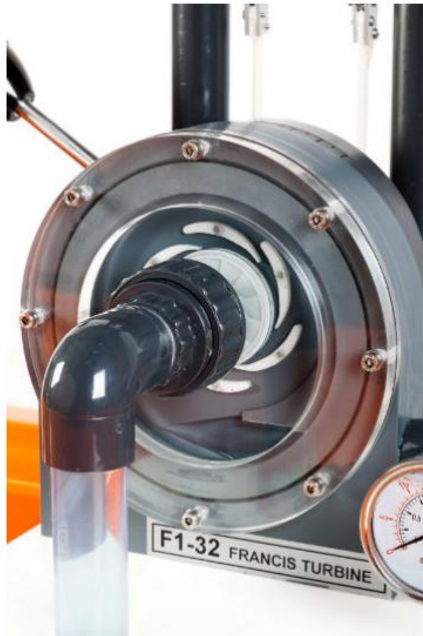
F1-32 Showing the runner and guide vanes behind the outlet to the draft tube
