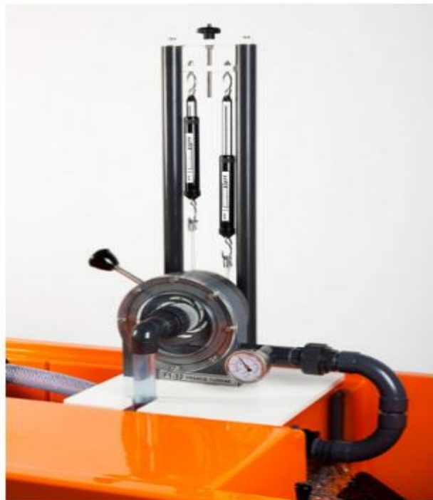
F1-32 Francis Turbine
